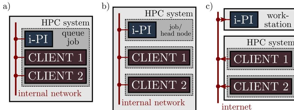
**Figure 2.1:** Different approaches to run i-PI and a number of instances of the forces code on a HPC system: a) running i-PI and the clients in a single job; b) running i-PI and the clients on the same system, but using different jobs, or running i-PI interactively on the login node; c) running i-PI on a local workstation, communicating with the clients (that can run on one or multiple HPC systems) over the internet.
