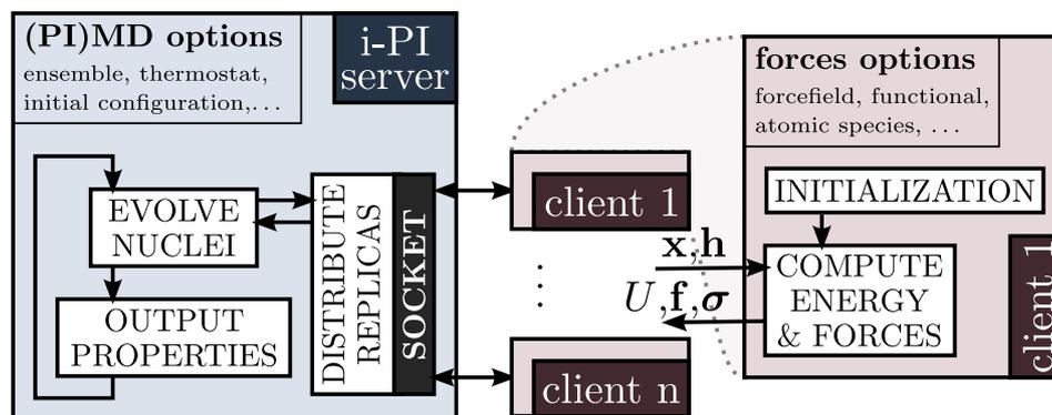
**Figure 1.1:** Schematic representation of the functioning of i-PI.
